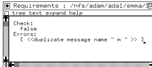
Figure 5: Result of checking a BMSC with a double occurrence of message m
