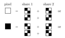
Figure 17: Visual crypto: the construction of shares.
