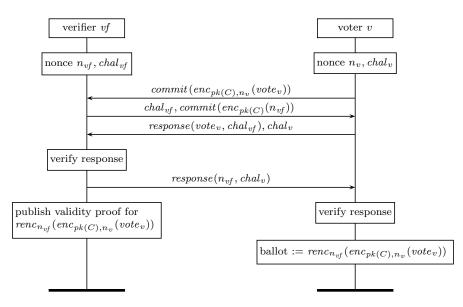
Figure 12: Verifier and voter jointly computing an encrypted ballot in LK00.
