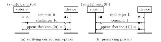
Figure 19: Verification and privacy of one bit-encryption in MarkPledge.
